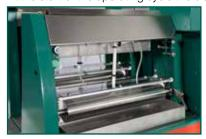
sition. A book block is opened in the centre, placed on the blade and pushed against the rear limit stop. The casing-in cycle is next triggered. The blade drives downwards between the gluing units.
