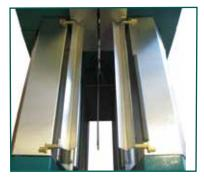
The machine control ensures that the spread of glue is slightly thicker in the joint area. The additional glue applied to the joint can be regulated independently of the normal spread thickness, thereby adjusting the glue level to suit the overlap of mull. The length of the additional gluing surface can also be set via the control unit, so that even widely overlapping mull represents no problem.
