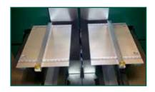
**Barcode reading system** - to secure the matching of book block and case. When the codes match, the casing-in process is activated automatically.
